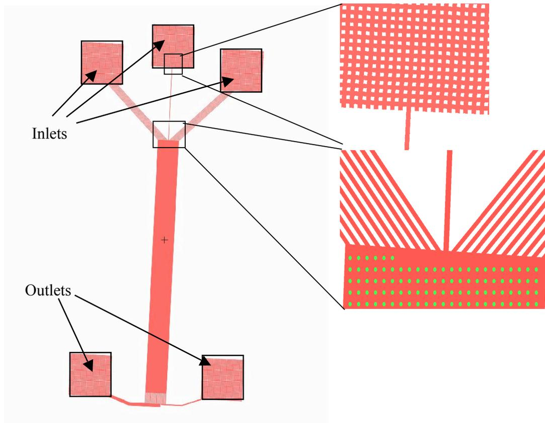
Figure 2.2. Design of the bumper array used in this project.
