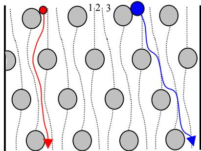
Figure 2.4. The streamlines and the way particles travel through a bumper array with  $N = 3$
