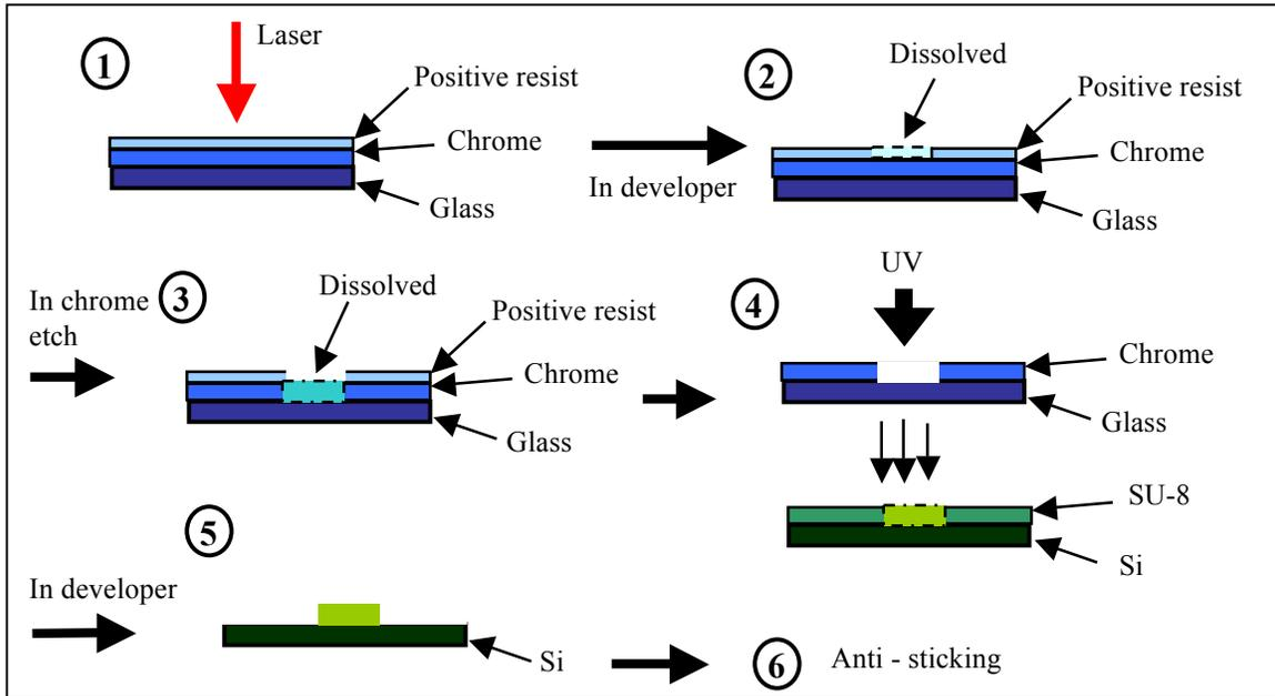
Figure 3.1. Show the process of master production.
