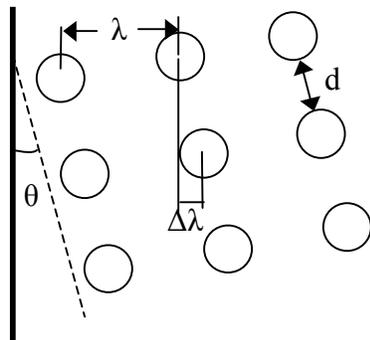
Figure 2.1. The Bumper array and how the posters are placed.[2]
