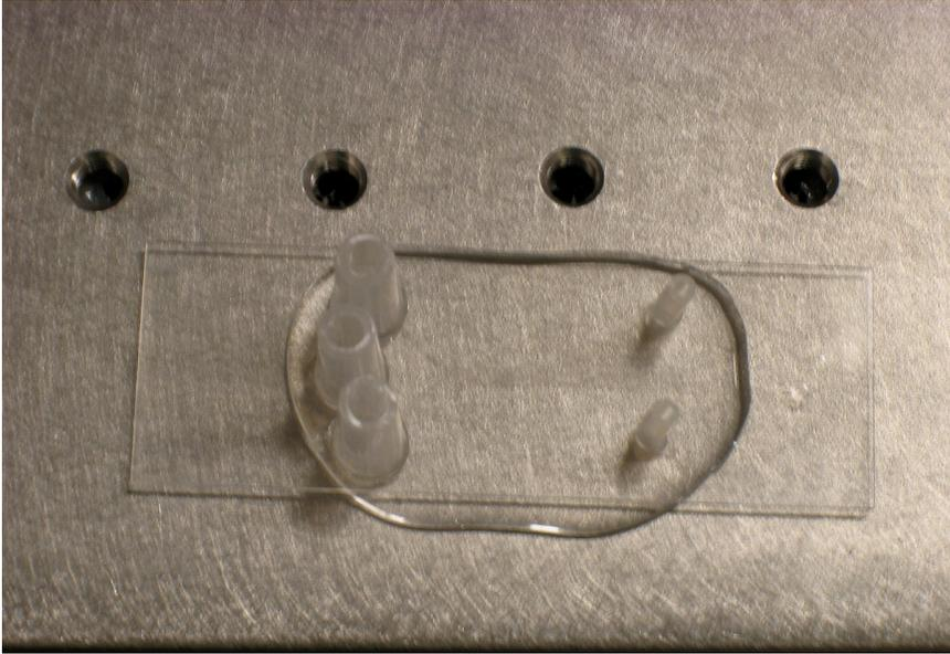
Figure 3.2. The whole device with the bumper array, glass cover and reservoirs.
