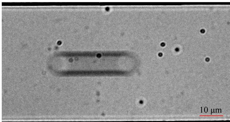
Figure 6.1. The outlet channel for bumped oil drops.
