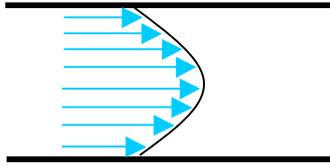
Figure 2.3. The Flow in the bumper array has a parabolic shape. [2]
