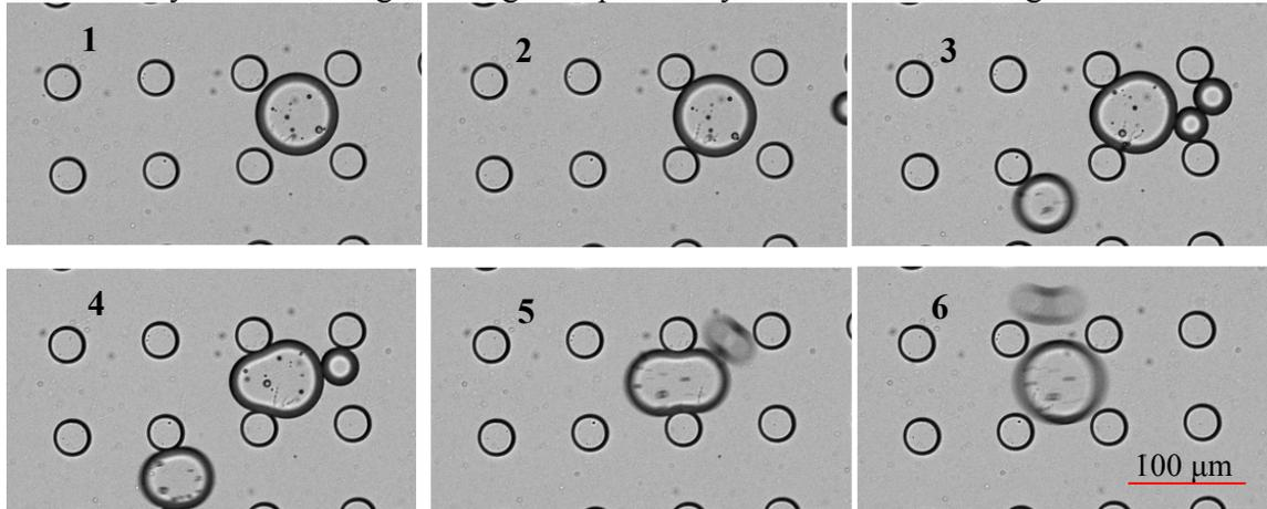
Figure 4.9. A big oil drop deforms itself to get past the post array.
