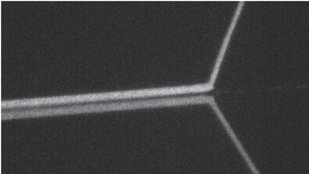
*Fig. 12 Stable laminar flows were obtained without pumping (each flow line is ca 20 microns wide). Buffer solution in the central flow keeps diffusing avidin and biotin labeled beads in the outer flows from aggregating before reaching the intersection where the optical tweezers transported beads can extract them.*
