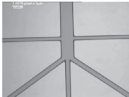
*Fig. 6 Microscope image of details of the Silicon SU-8 masters showing structures for casting the channel intersections.*
