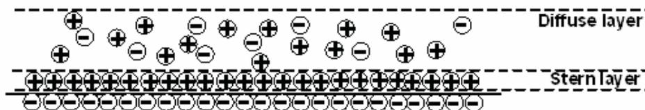
Fig 1. Schematic of the configuration of charges in a channel under electroosmotic conditions showing the mobile charges in the diffusive and fixed charges in the Stern layer.
