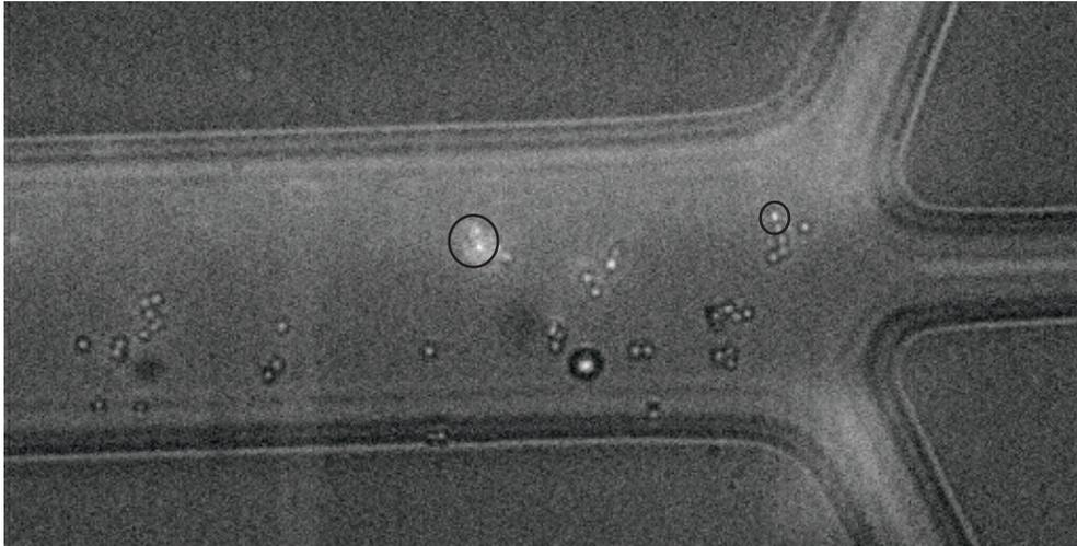
*Fig. 14 Optical trapping of avidin covered micronsized beads were achieved but unspecific adhesion to the roof of the channels inhibited device function. Shown are a number of beads that were immobilized after trapping. Binding to fluoresescently labeled 40 nm biotinylated beads can be seen on the avidin beads immobilized closest to the upper third of the channel where the laminar flow of biotinylated beads is. (Encircled in image)*
