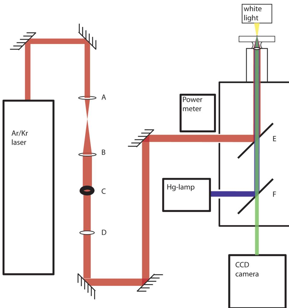
*Fig. 9 The setup of the optical tweezers housed in the microscope. The laser is guided through the beam expanding lenses (A) and (B) and subsequently passes an aperture (C) and a band pass filter (D) filtering out the undesired laser wavelengths. A dichroic mirror (E) reflects the laser onto the back of the objective overfilling it. Another dichroic mirror (F) guide the UV-light into the objective.*
