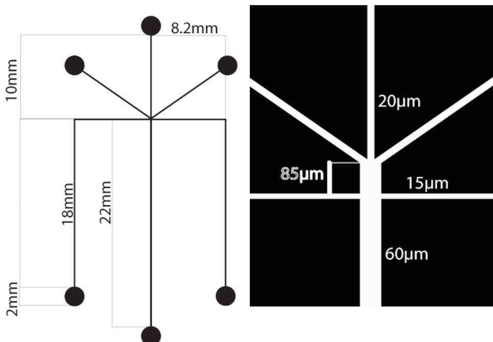
Fig. 5 The final design of the photomask (left) and channel intersections in detail (right)
