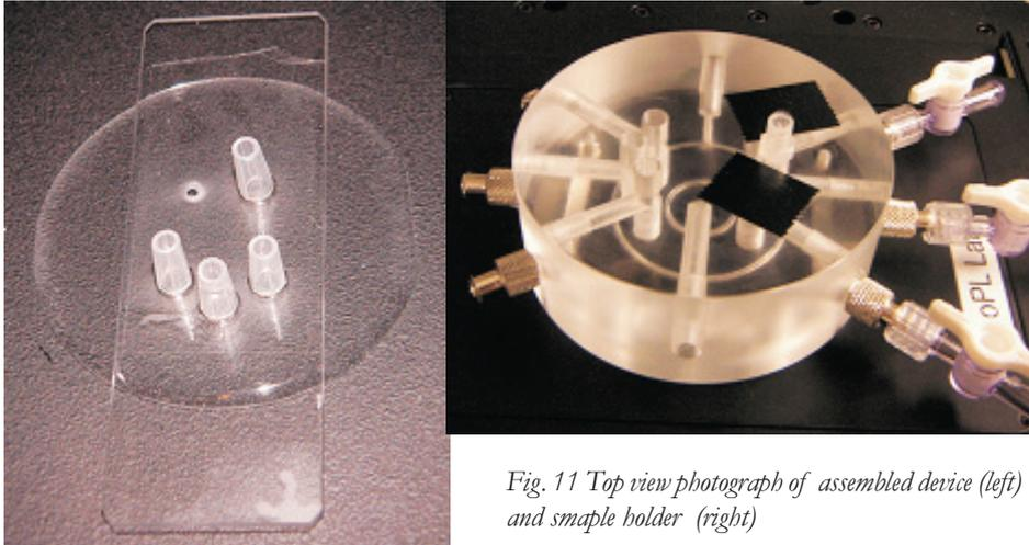
*Fig. 11 Top view photograph of assembled device (left) and sample holder (right)*
