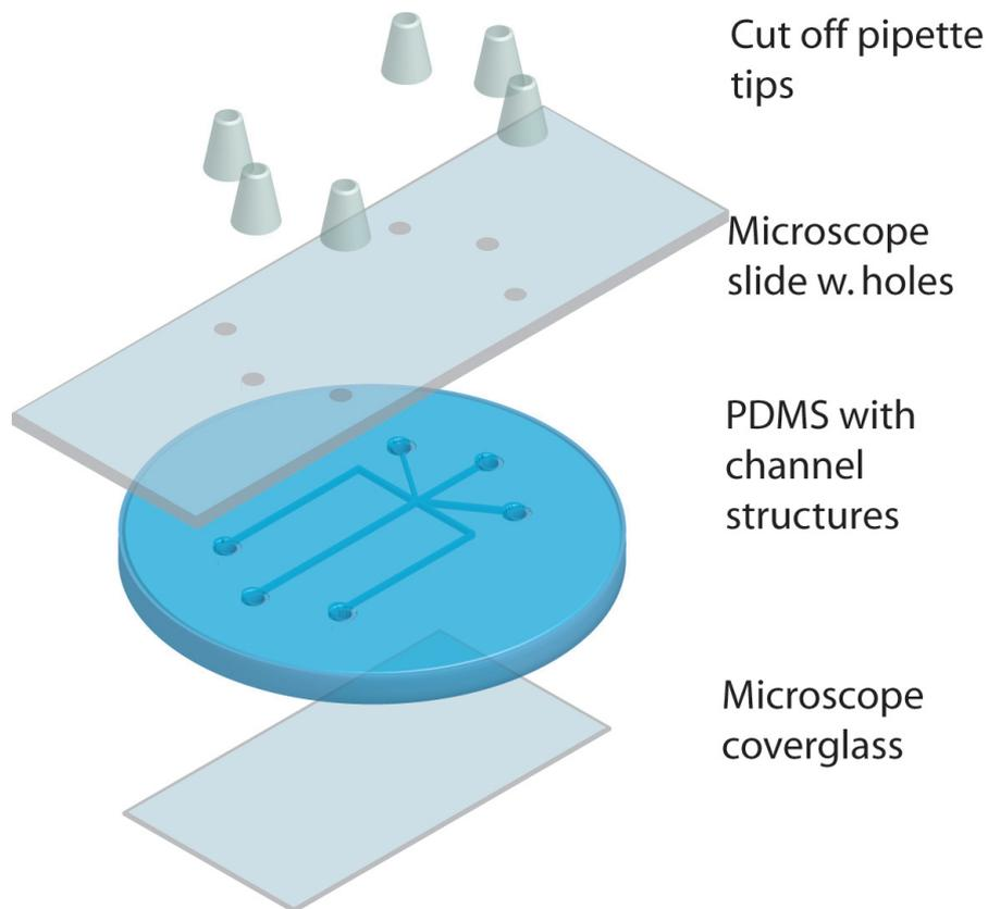
*Fig. 8 Schematic view of the final assembly of the microfluidic device. PDMS and glass slides were irreversibly bonded using an oxygen plasma and cut off pipette tips were glued to the device using optical adhesive.*
