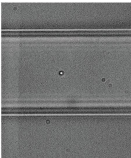
*Fig. 13 Manipulation of optically trapped 1 micron sized beads were performed in the microfluidic channels.*
