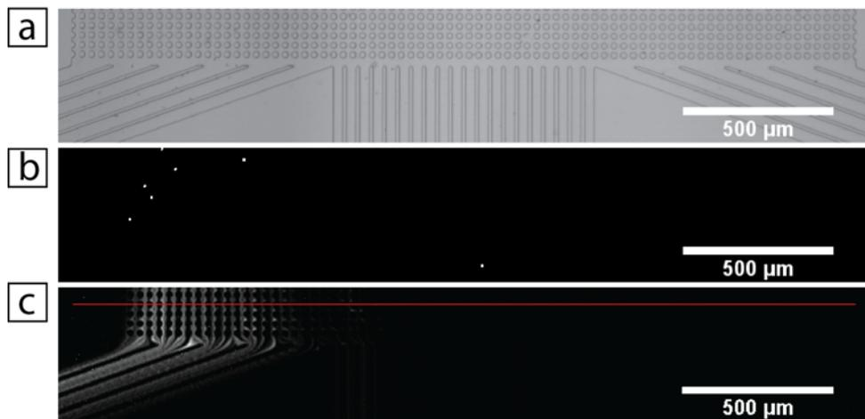
**FIGURE 7.10.1:** Image analysis of outlet trajectories. (a) Single image frame from a video captured with a high-speed camera. (b) Frame from (a) which first has had its static background subtracted and then been converted to a binary format at a grayscale pixel threshold with no noise. (c) Sum of 15 000 frames processed like that in (b). Red line marks the location of where the pixel intensity was extracted.
