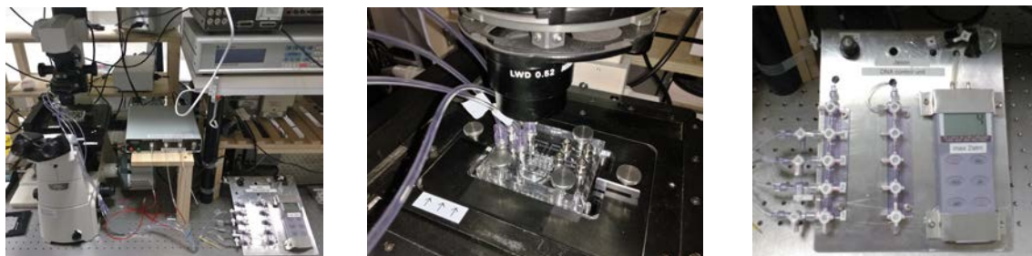
Figure 3.7: Images of the nanochannel setup featuring an overview image ( left ), the chip mounted on the microscope stage ( center ) and the pressure control system ( right ).
