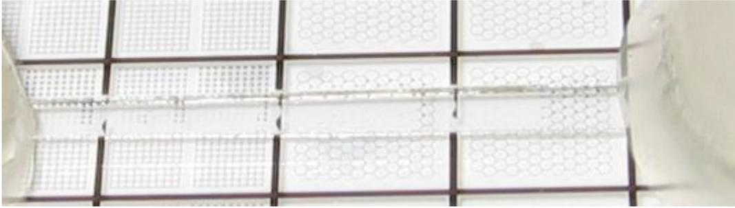
Figure 43: The places where the chrome has been dissolved is clearly visible.
