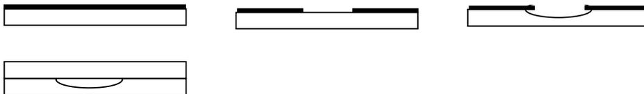
Figure 5A-B: An etch mask is applied and patterned. C: The glass is etched. D: Etch mask is taken away and the wafer is thermally fused with a flat glass.
