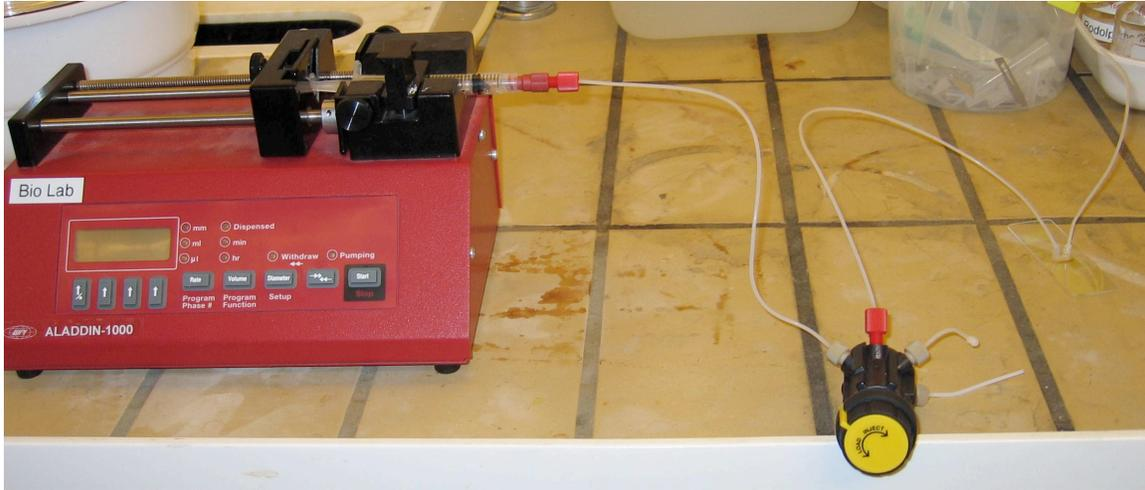
Figure 18: A loop system in between the pump and cell to get rid of bubbles during exchange of syringe (exchange of solution)
