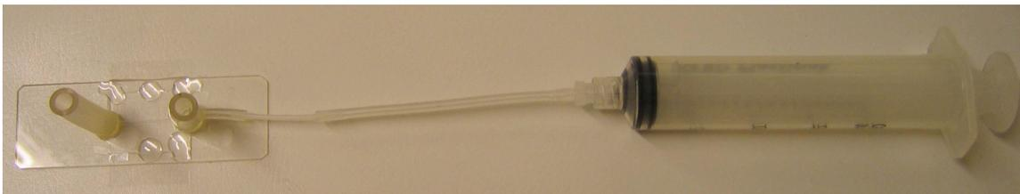
Figure 24: Solution is sucked by hand through the channel.
